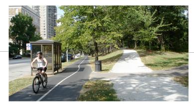
Multi-use paths are off-street bike facilities that are designed to accommodate bicyclists and pedestrians. Multi-use paths can be placed adjacent to a street and take the place of a sidewalk or be completely separated from a street, such as along a greenway. Off-street bikeways can be combined with on-street bikeways on any roadway type.
